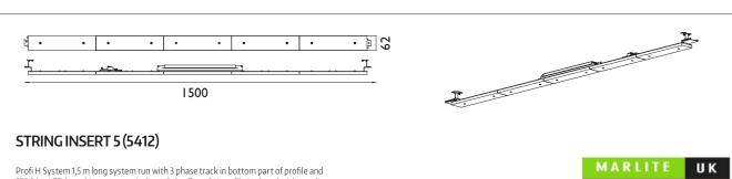
Profi H System 1,5 m long system run with 3 phase track in bottom part of profile and 5500 lm LED board in top part - indirect light. Top of H profile is closed with acrylic cover. Profile run can be used as part of profi H system and is equipped with line connectors and ceiling suspension system (1,5 m in standard, other lengths in request).
